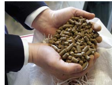
Pellets directly from the pieces of a kraft lignin cake
