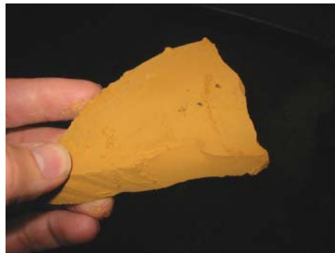
High quality lignin extracted from black liquor (kraft pulp mill)
