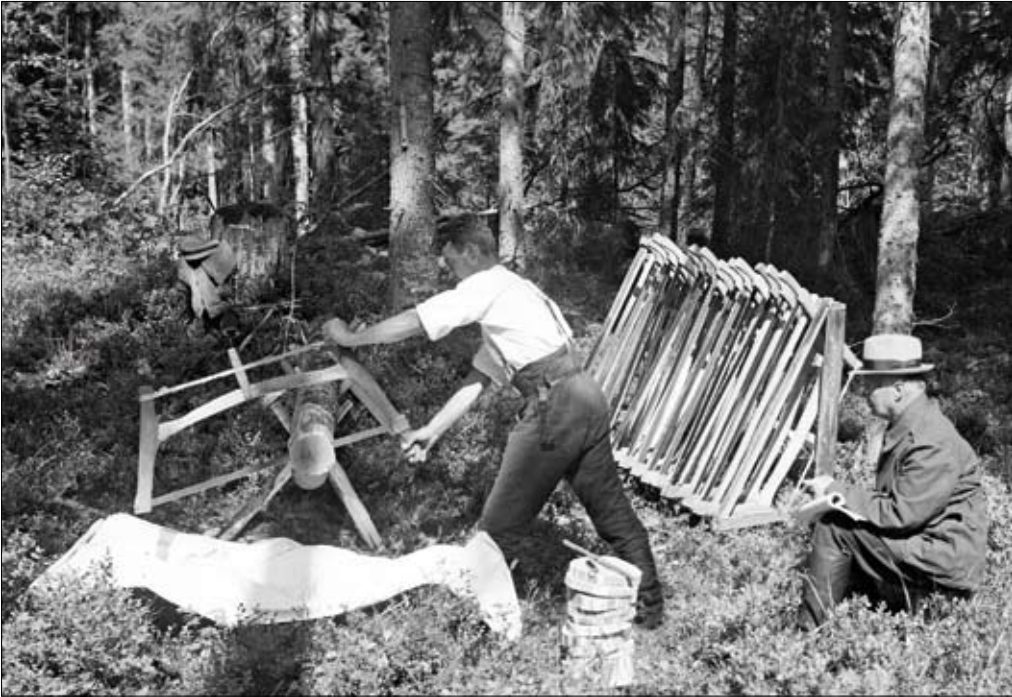
Photo 3. Bucking a tree by one-man manual saw of wooden frames, which was used for small trees. Work efficiency study is going on in the 1930s.
