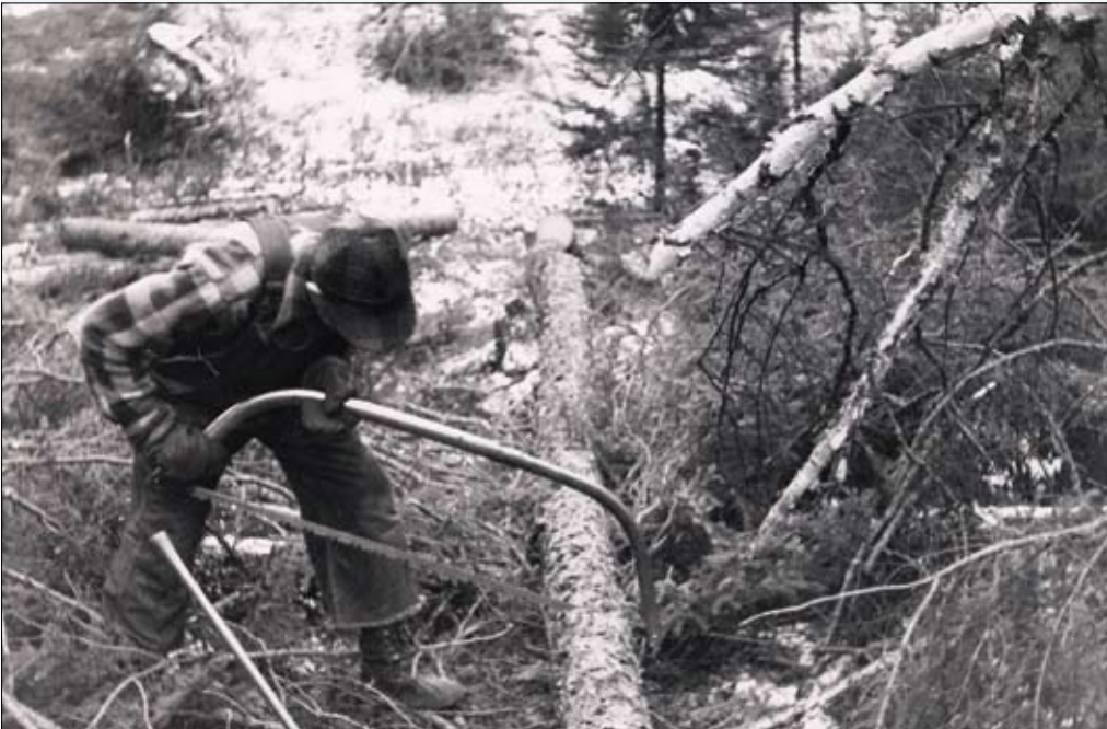
Photo 4. Bucking a tree with steel-framed manual saw in the 1950s.
