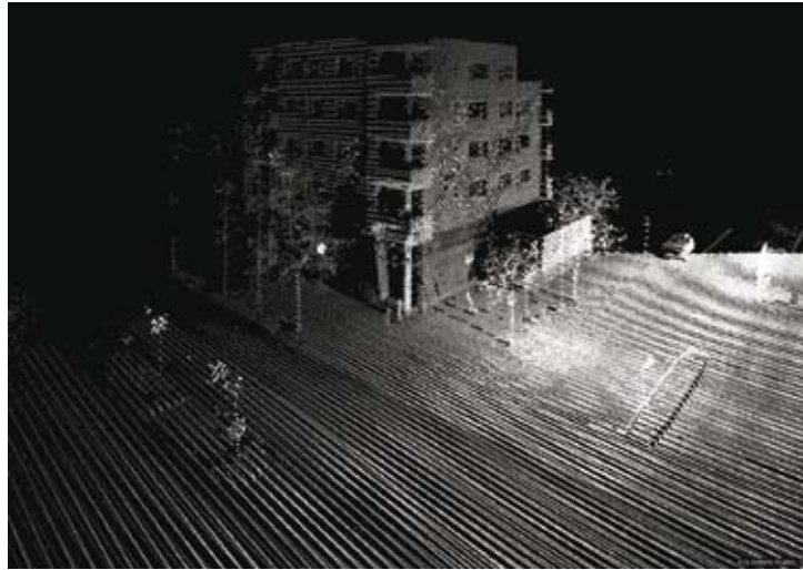
Figure 9.7 Representation of a point cloud collected with VLS from a city area. City trees are well characterised (Copyright Antero Kukko, Finnish Geodetic Institute).
