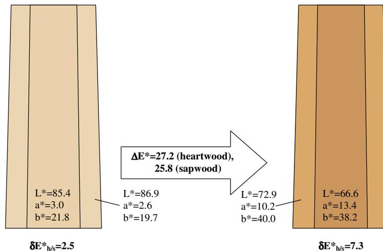
Fig. 6. The average wood colour parameters before and after the 2664 hours exposure of UV-A radiation (peak wavelength 340 nm).  $L^*$ =lightness,  $a^*$ =redness,  $b^*$ =yellowness,  $\delta E^*_{h/s}$ =colour difference between heartwood and sapwood,  $\Delta E^*$ =total colour change during the exposure.
