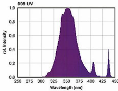
**Figure 2 :** Relative spectrum of the UVA-351 type fluorescent lamp (Narva LT 36W/009 UV).
