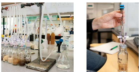
Fig. 3. Analyses: (1) Accumulated CO 2 by gas chromatography. (2) Recover of extracellular enzymes by centrifuging method. (3) Enzyme activity assays of four glycoside hydrolases (β-glucuronidase, β-xylosidase, β-glucosidase and cellobiohydrolase) by fluorimetric method. (4) Amplification of total fungal DNA with primer-pair ITS1F-GC and ITS2 and separation by DGGE.
