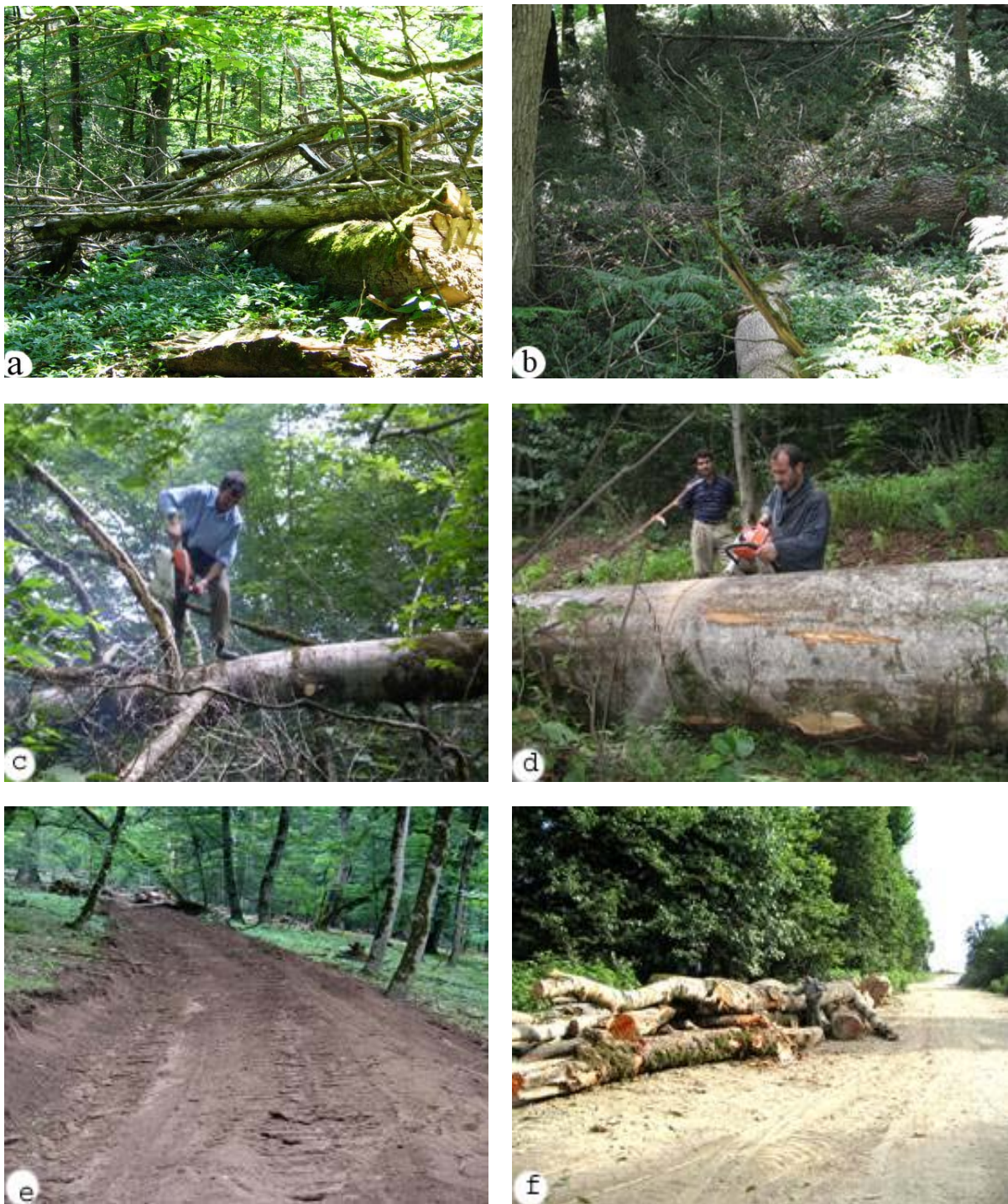
Figure 6. Typical conditions of wood procurement in Iran. a) Felled tree in the forest, plenty of time should be consumed for clearing (or cleaning) along the stem of cut tree; b) Ground condition and felled tree ready for processing; c) delimiting and topping is done in dangerous position; d) performance of cross-cutting of Fagus orientalis ; e) prepared skid trail for skidding; f) roadside landing.
