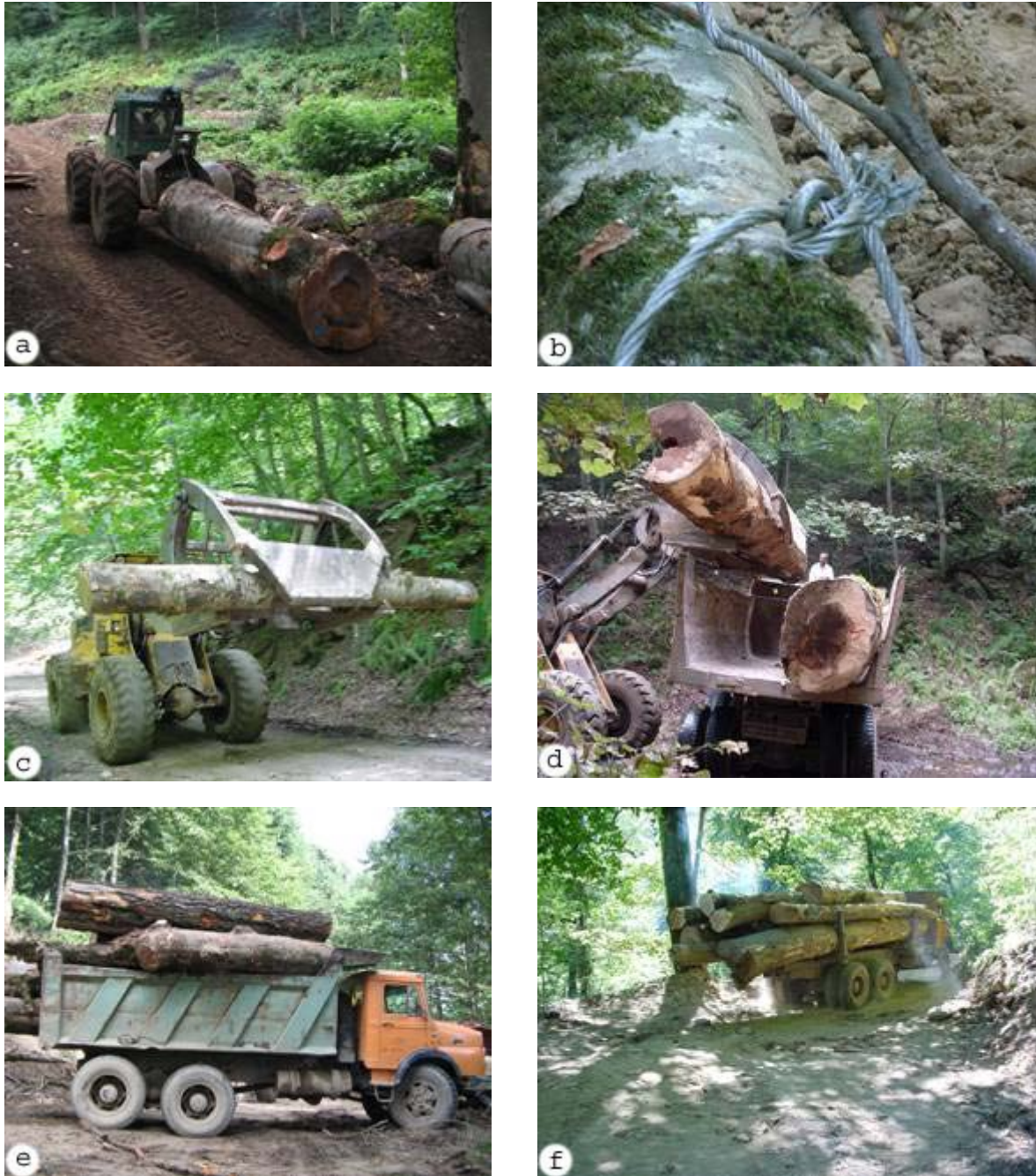
Figure 7. Primary and secondary transportation in Iran: a) wheeled skidder, equipped with cable, skidding the log; b) hooking of log; c) front-end loader carrying the log for loading; d) loading performance at the roadside landing by loader; e) dump-truck used for carrying short-log; f) special truck for long-log.
